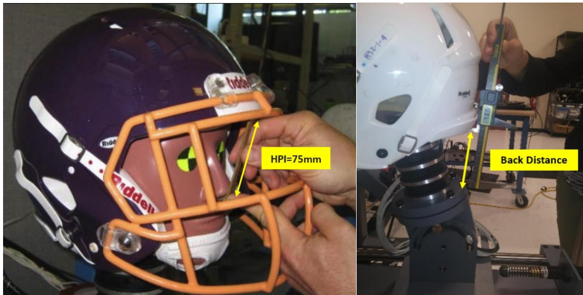
Figure 3. Demonstration of the use of the nose gauge and helmet positioning index (left). A secondary measurement (back distance) between the center of the lower back of the helmet shell and the neck base may be measured using calipers to ensure that the helmet is seated on the head repeatably (right).
